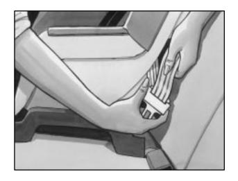
Tilt the latch plate to adjust the belt if needed.If the shoulder belt goes in front of the child's face or neck, put it behind the child restraint.
